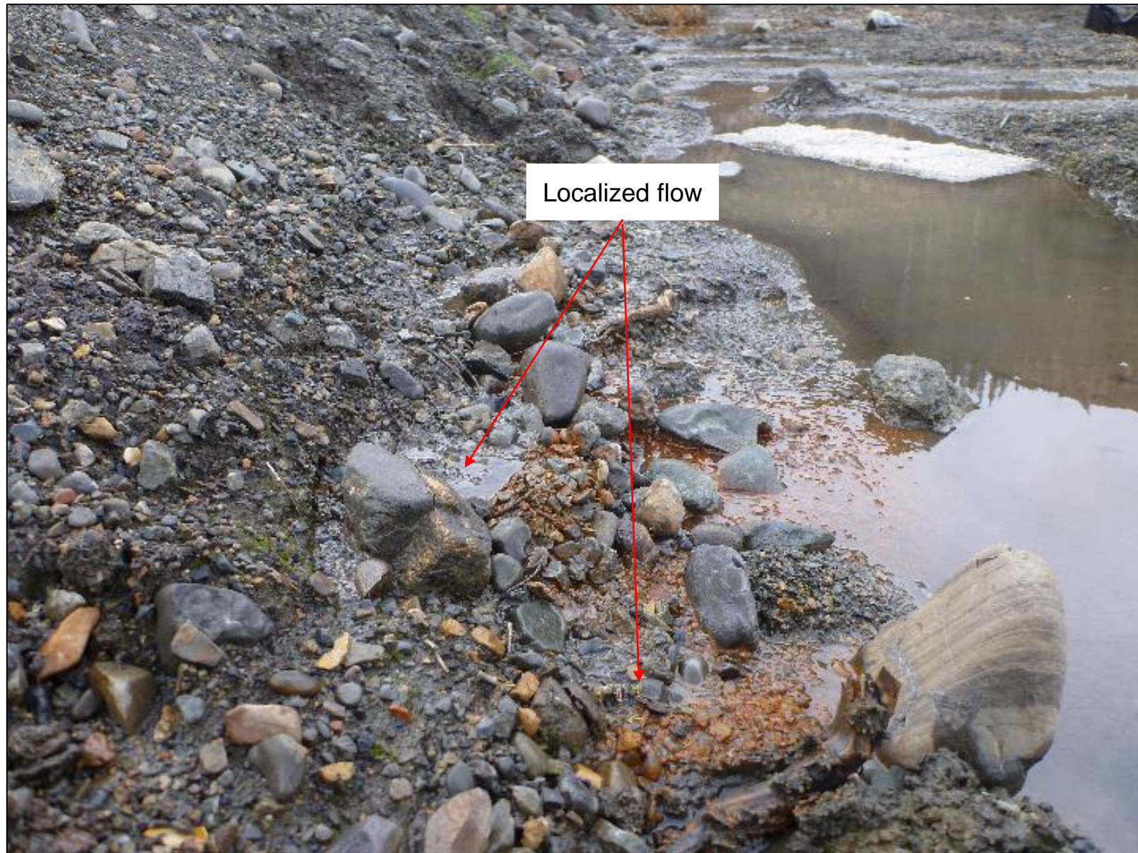
Chainage 0+250: Localized flow (~0.25 L/min), noted in Photo 4. Looking west.
