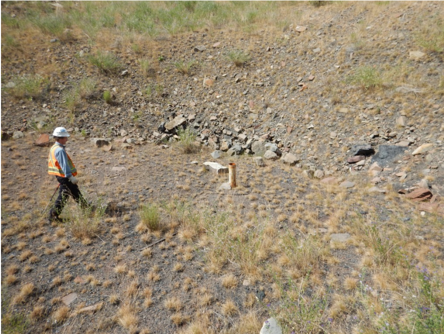
Photo I-10 P96-1 and P96-2 surface casing. No piezometer cables accessible in casing.
