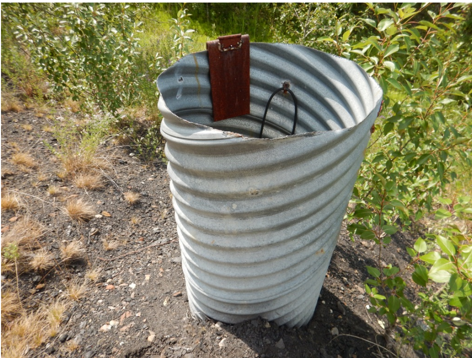
Photo I-15 Pneumatic piezometer leads (x3) at downstream toe of embankment. Sta. 0+475 readings collected during 2014 DSI. (PS-2014-26)
