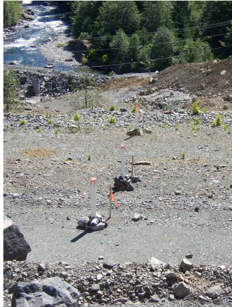
B) Survey markers to measure settling on the TDF
