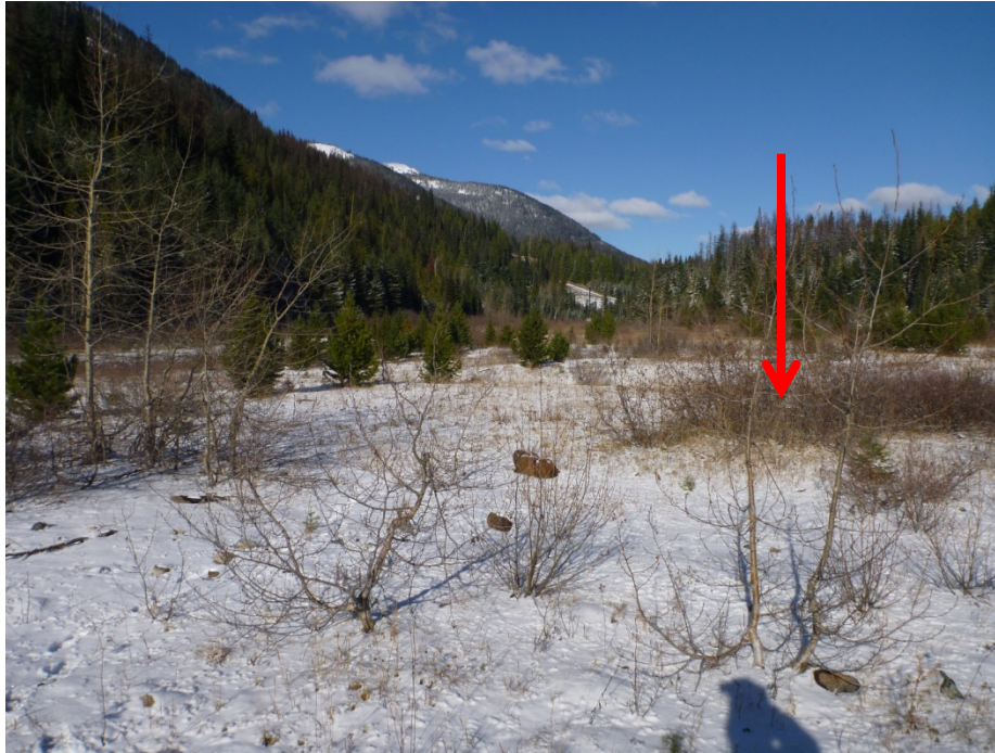
Photo 55 – Jumbo reclaimed tailings surface. Photo taken facing north. Red arrow indicates depression located near site of 1998 sinkhole where tailings were transported under dam through corrugated metal pipe passing beneath tailings impoundment.
