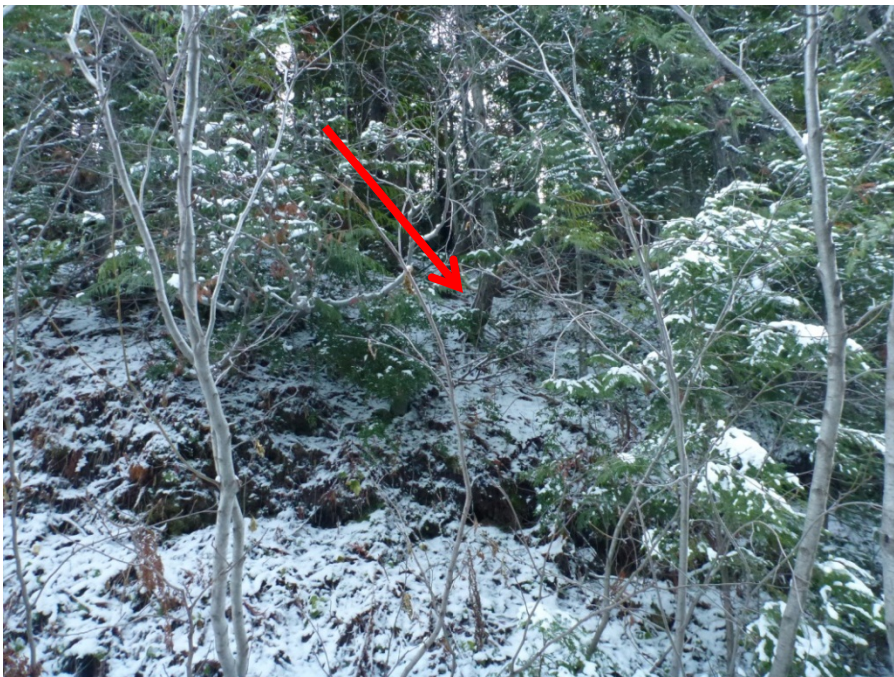
Photo 30 – Good Friday West Limb, downslope of downstream toe area. Photo taken facing east from access road from Hwy 3B. Natural slope between access road and downstream toe of West limb shows signs of surficial instability, possibly associated with the cut slope for the road. Red arrow indicates tree with bent trunk associated with slow movements of slope surface.
