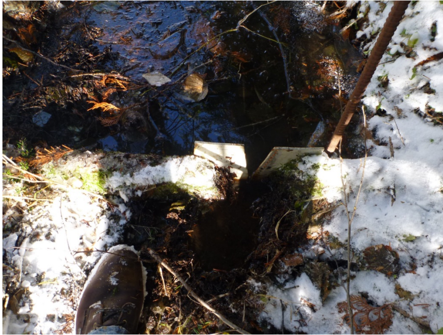
Photo 33 – Good Friday v-notch weir at seepage monitoring and sampling Site 18. Weir has become clogged with leaves and organic matter since initial installation.
