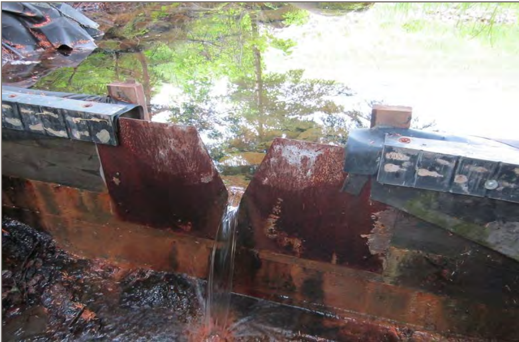
Photo 8: V-notch weir located downstream of the east embankment to measure seepage estimates
