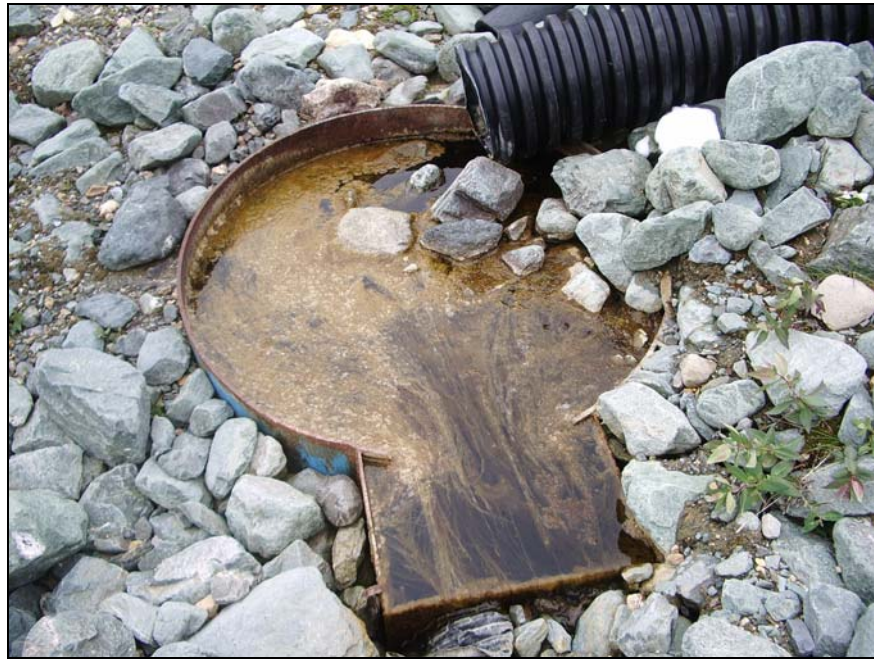
PHOTO 9 – Water Flow from Fleece Bowl Heap Leach Facility V-Notch (Looking South)
