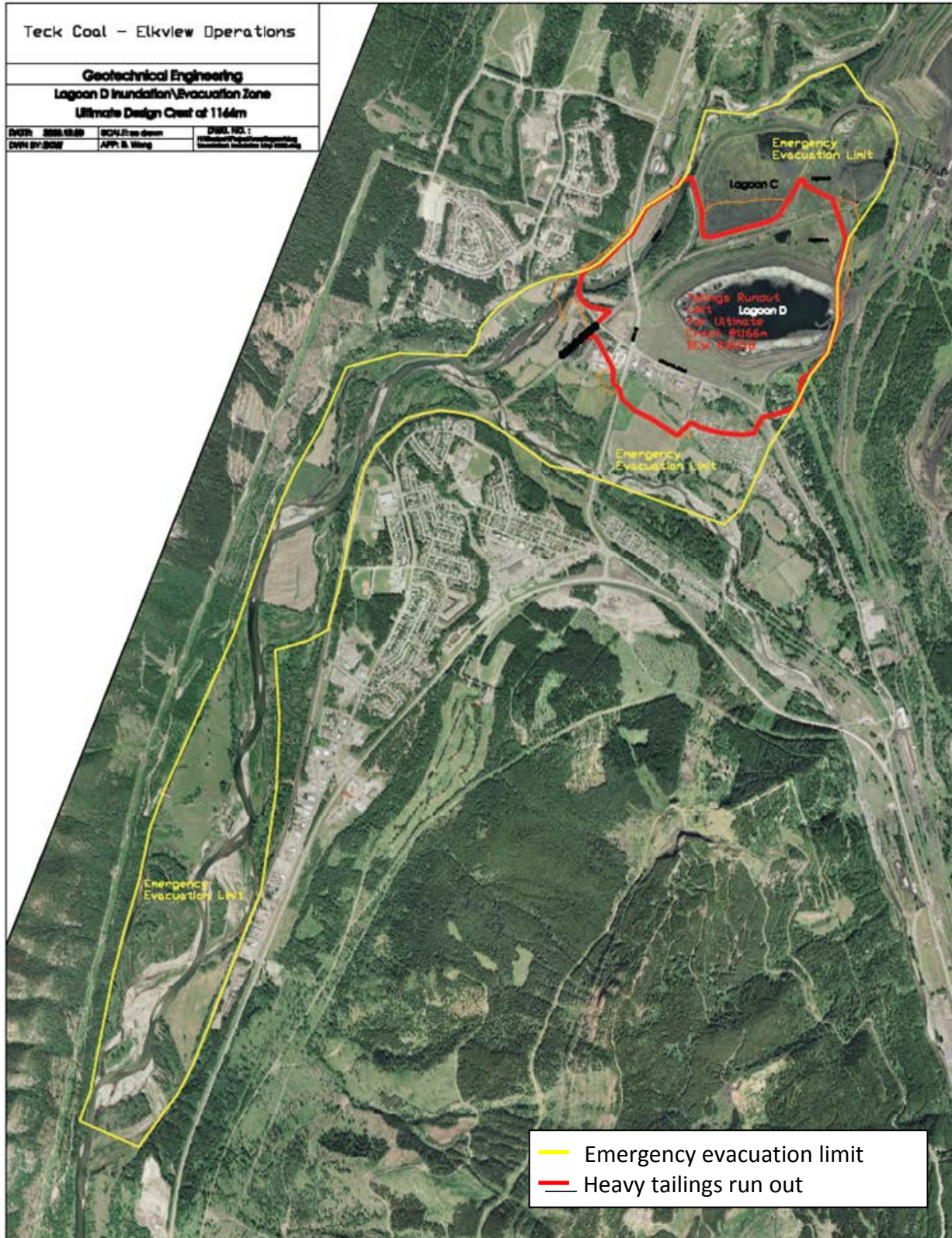
Figure 5: Inundation Area and Evacuation Limit
