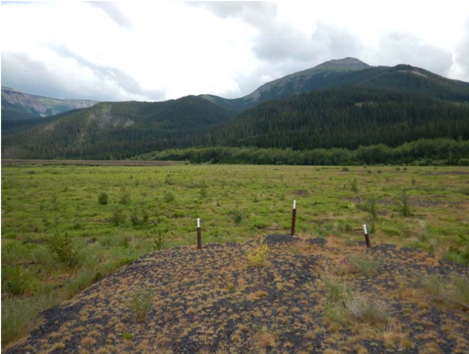
Photo I-10 Piezometer standpipes (PC1, PC2, PC3) in tailings beach. (TSF-2014-01)
