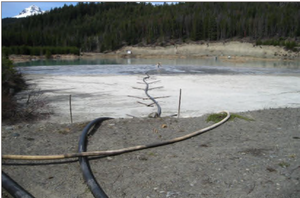
Photo 12: Tailings discharge – line partially buried (maintenance required)
