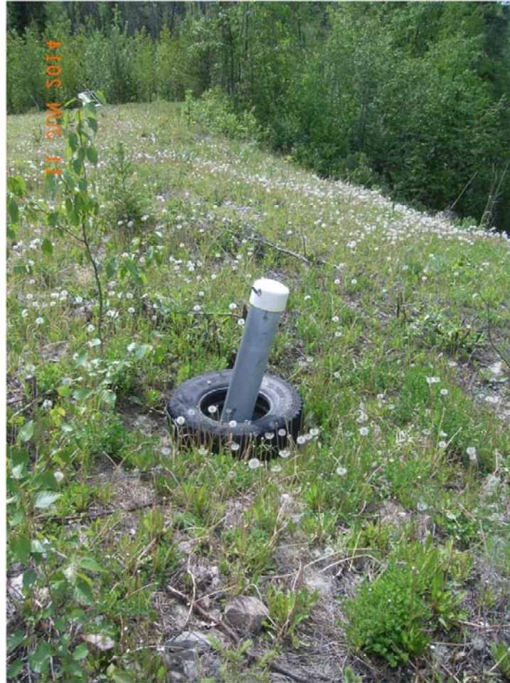
Photo D6-4: Close up view of the crest of dam showing protective casing around standpipe monitoring well. The monitoring well is located on the downstream slope, mid-way along the dam. Looking east. Note that the protective casing and the standpipe were broken. (11 June 2014)
