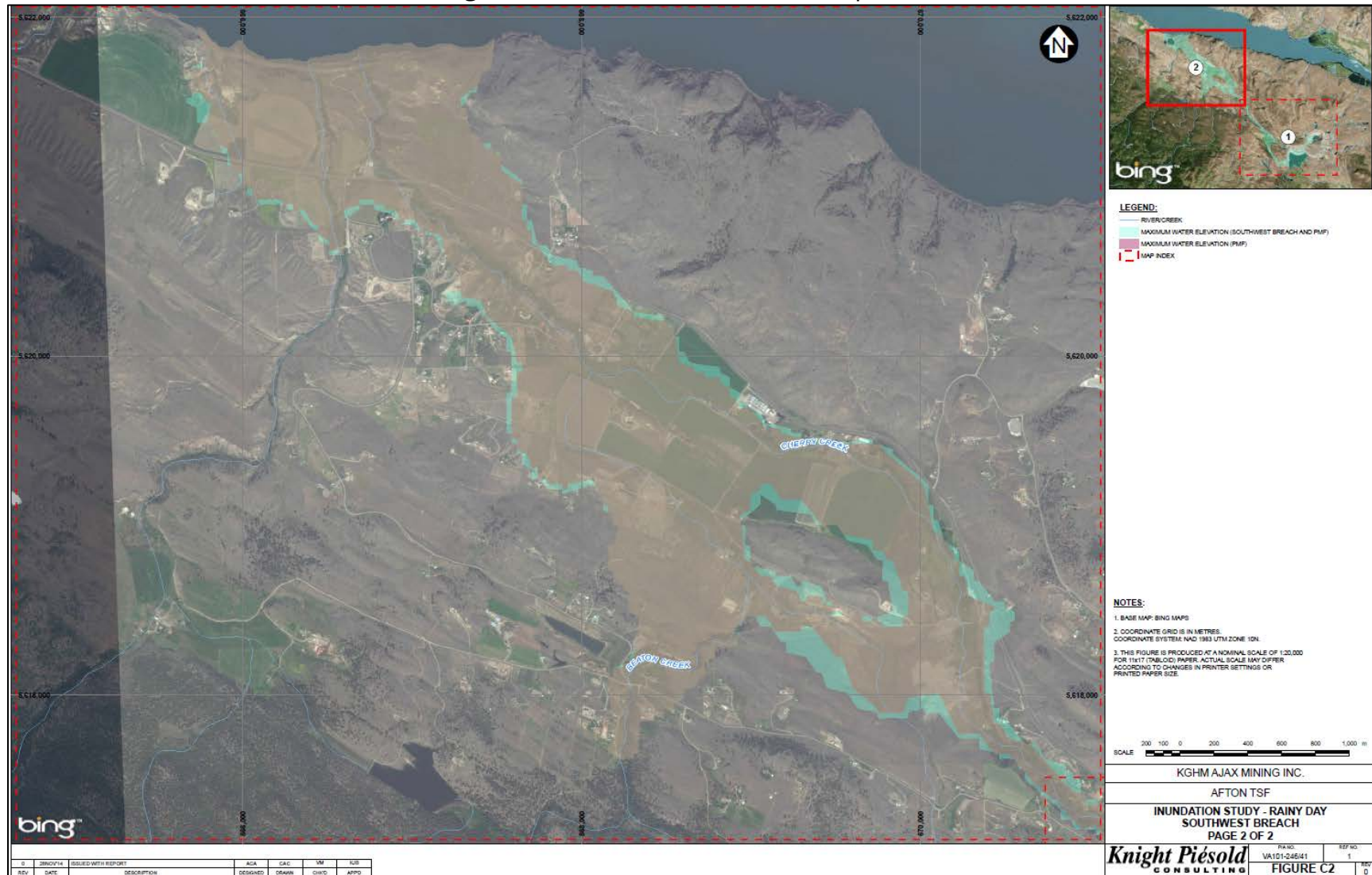
Figure 7: West Dam Inundation Map No. 2
