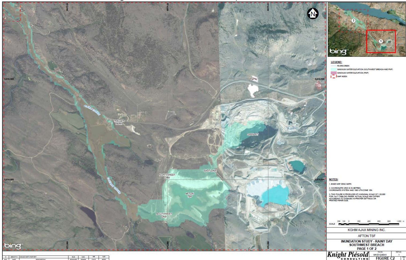
Figure 6: West Dam Inundation Map No. 1
