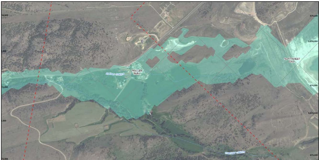
Figure 2 West Dam, Northwest "Sunny Day" Failure – Inundation Map at Trailer Park
