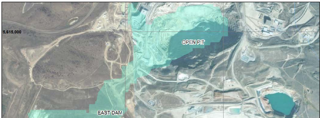
Figure 3 East Dam Failure – Inundation Map
