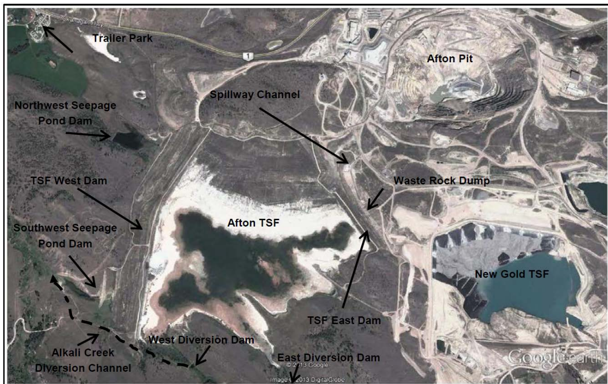
Figure 1 Afton TSF General Arrangement
