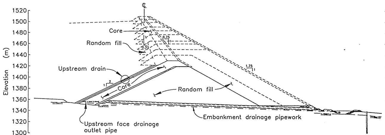
Figure 8 Typical section through Kemess South embankment
