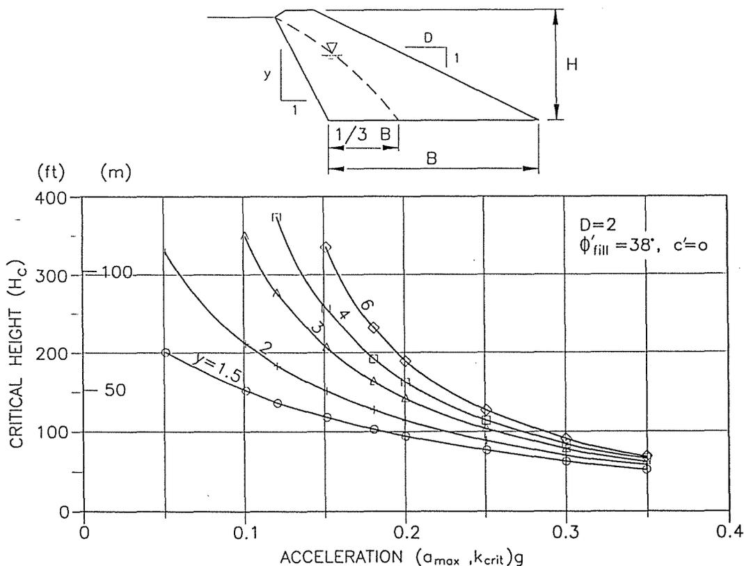
Figure 4 Relationship between critical height and acceleration
