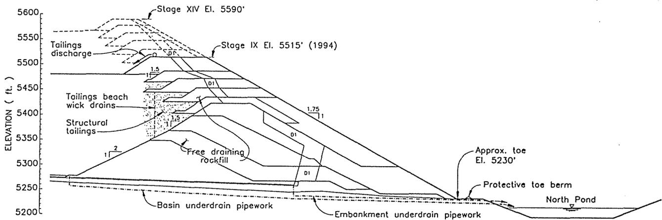
Figure 6 Typical section through Montana Tunnels embankment
