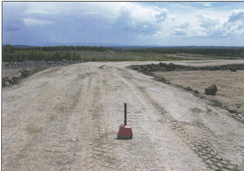
PHOTO 8 – Using the nuclear densometer to confirm field densities of Zone S material.
