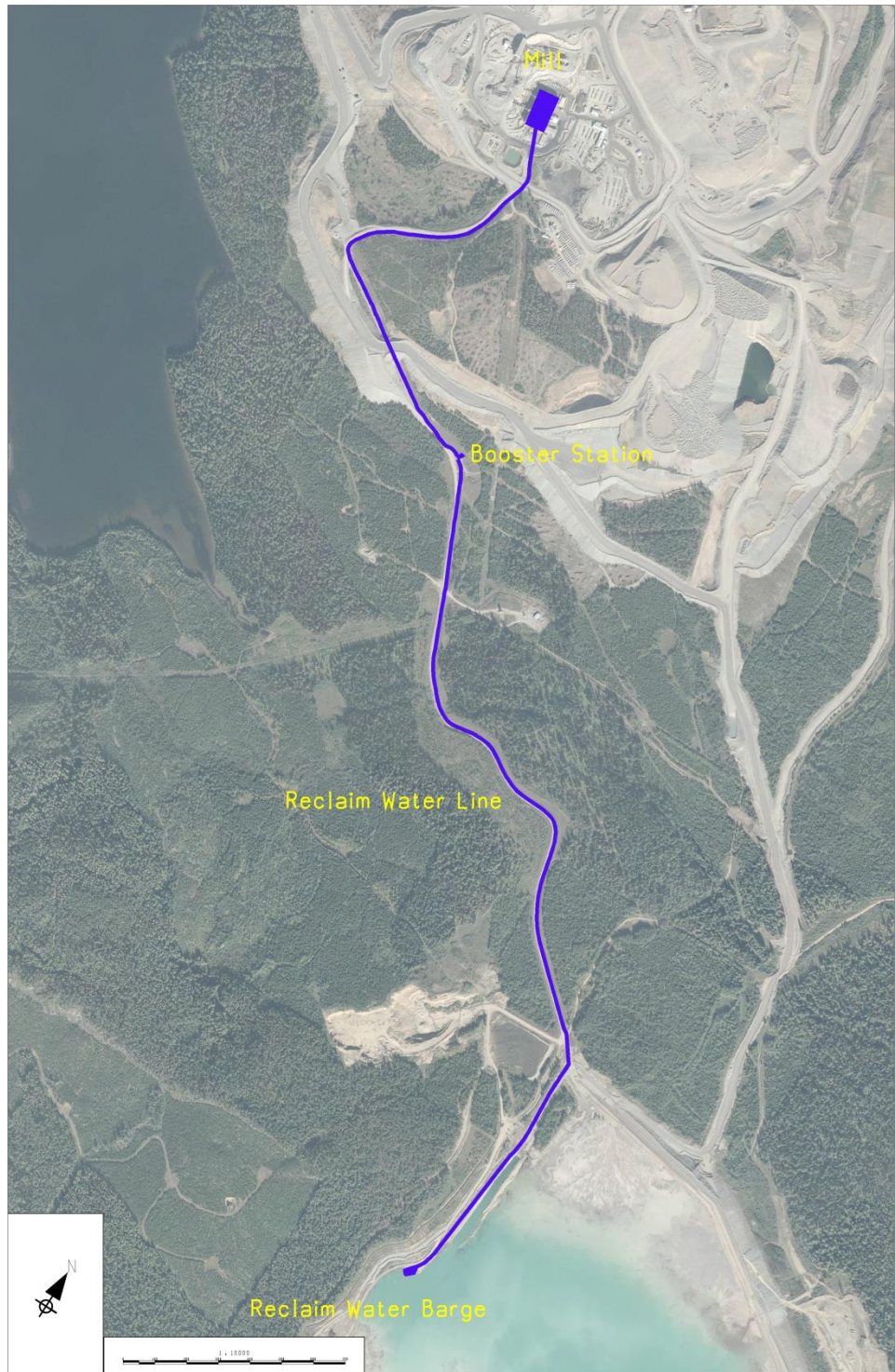
Figure 5.1.1.18.1 – Reclaim Water System
