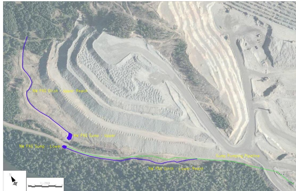
Figure 5.1.1.2.1 - NW PAG Ditch and Sump System
